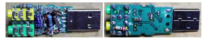
'3D Sound' soundcard with soft-clip circuit modifications as shown in schematic below.
