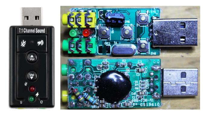
'7.1 Channel Sound' virtual soundcard with just the basic modifications shown in schematic below (no protection clipper parts). The circuitry appears to be fairly similar to the '3D Sound' device, and is modified in the same manner.
